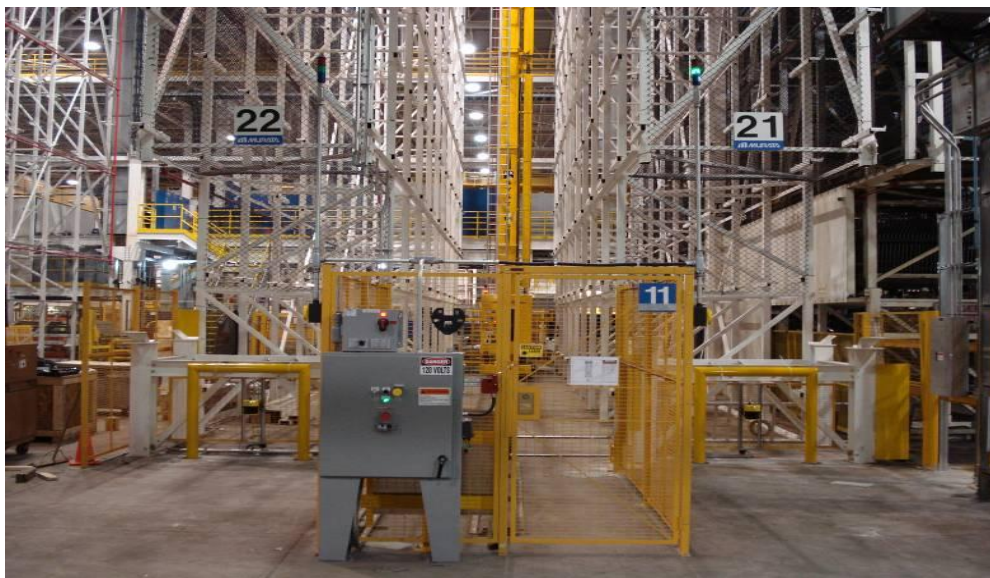
Chrysler AS/RS Aisle with Category 3 Dual Channel Safeties and ANSI Z244.1 Compliance
